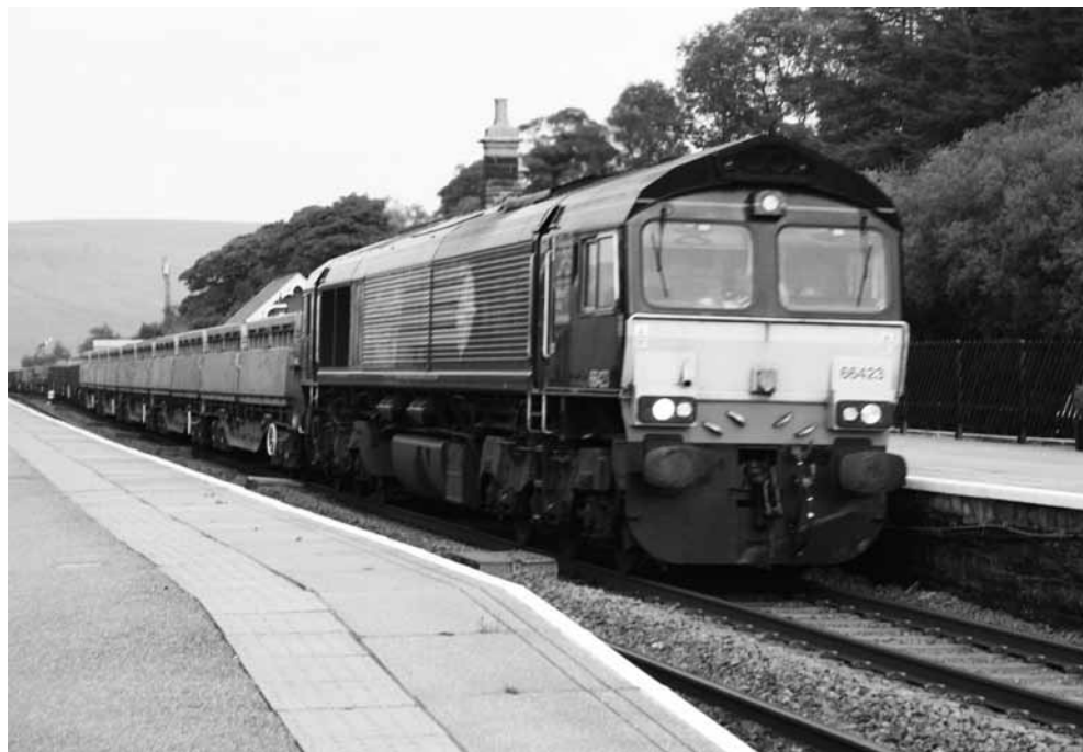
66423 with a rake of wagons including MRA bogie side tip ballast wagons and MHA 4-wheel ballast/spoil open box wagons. Seen at Garsdale station. Photo: Roger Templeman
